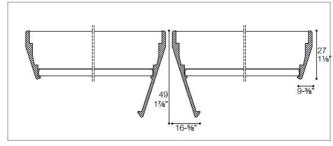
In the case of pairs of doors, grip is ensured on both sides.
