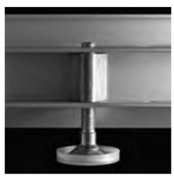
Adjustment and levelling foot with a capacity of 100-37%" kg. The adjustment is transmitted along the entire length of the frame in order to avoid imbalances typical of traditional wardrobes with wooden base. The possible adjustment is from 0 to 12mm-1/2"1.
