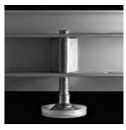
Adjustment and levelling foot with a capacity of 100-31/8" kg. The adjustment is transmitted along the entire length of the frame in order to avoid imbalances typical of traditional wardrobes with wooden base. The possible adjustment is from 0 to 12mm-1/2"1.
